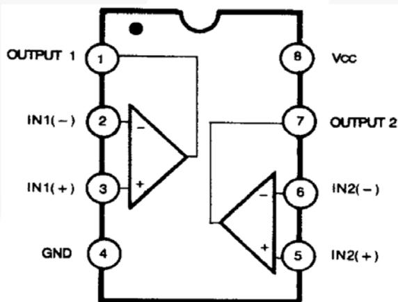
Figure 3. Block Diagram
