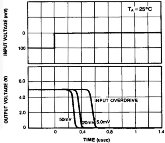
Figure 8. Response Time for Various Input Overdrive-Negative Transitions
