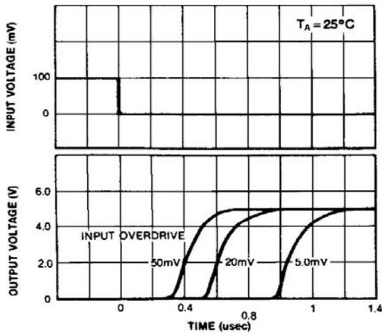
Figure 9. Response Time for Various Input Overdrive-Positive Transitions
