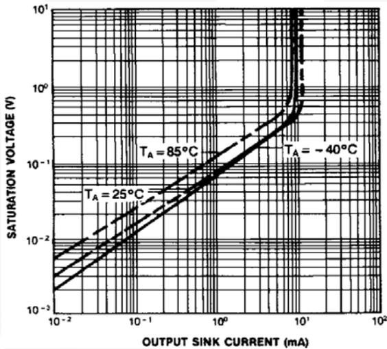
Figure 7. Output Saturation Voltage vs. Sink Current
