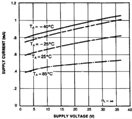
Figure 5. Supply Current vs. Supply Voltage
