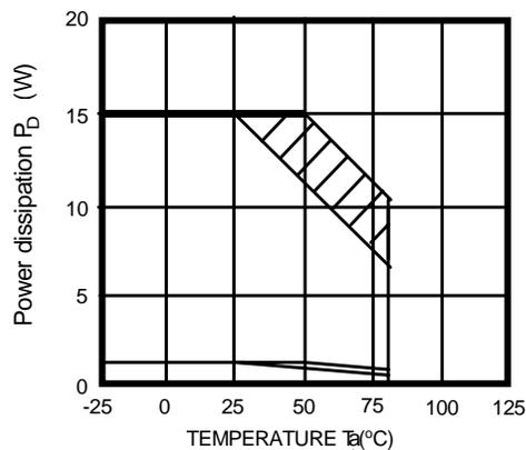
**Figure 7. Power Dissipation vs. Temperature( $T_a$ )**
