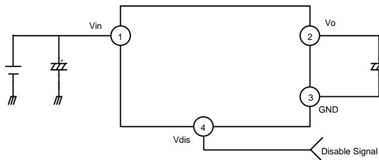
**Figure 1. Application Circuit**
