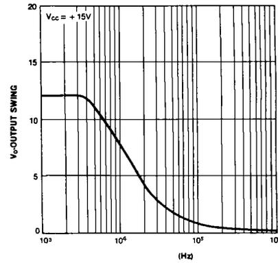
Figure 4. Large Signal Output Swing vs Frequency
