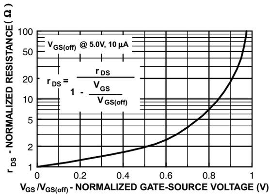
Figure 7. Normalized Drain Resistance vs. Bias Voltage
