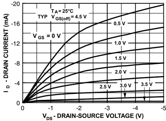
Figure 3. Common Drain-Source
