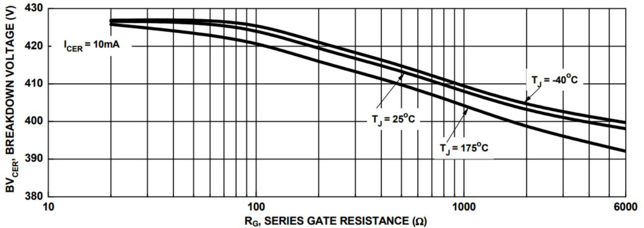
Figure 15. Break Down Voltage vs. Series Resistance
