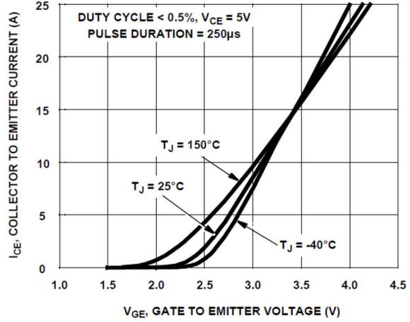
Figure 8. Transfer Characteristics
