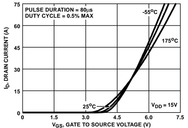
FIGURE 8. TRANSFER CHARACTERISTICS
