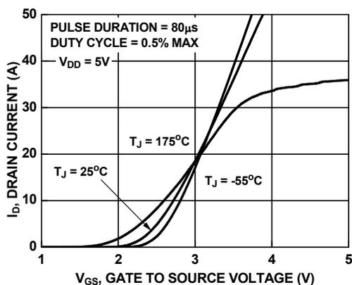
Figure 7. Transfer Characteristics
