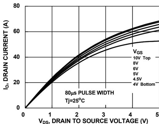
Figure 9. Saturation Characteristics
