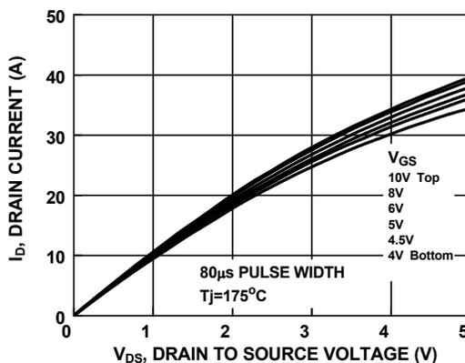
Figure 10. Saturation Characteristics
