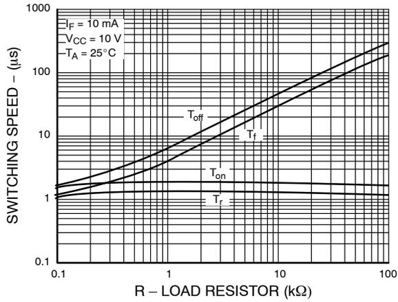
Figure 7. Switching Speed vs. Load Resistor
