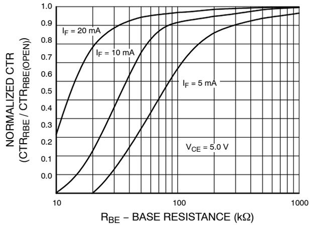
Figure 4. CTR vs. RBE (Unsaturated)
