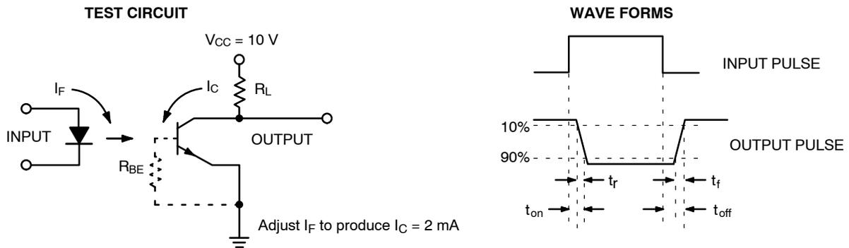
Figure 11. Switching Time Test Circuit and Waveform
