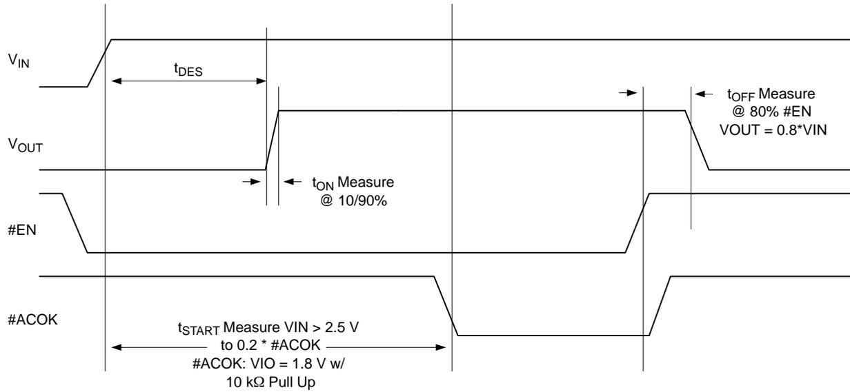
Figure 3. Timing for Power Up and Normal Operation
