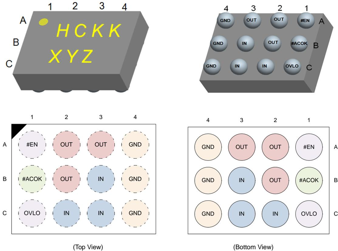
Figure 2. Pin Configuration
