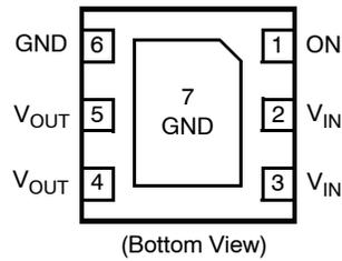
**Figure 3. Pin Configuration**
