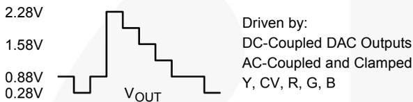
There is a 280mV offset from the DC input level to the DC output level.  $V_{OUT} = 2 * V_{IN} + 280mV$ .
