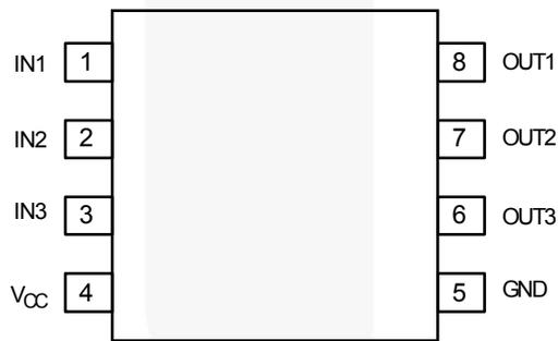
Figure 2. Pin Configuration
