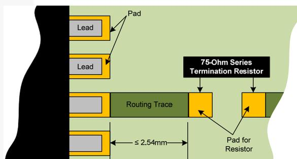
Figure 13. Termination Resistor
