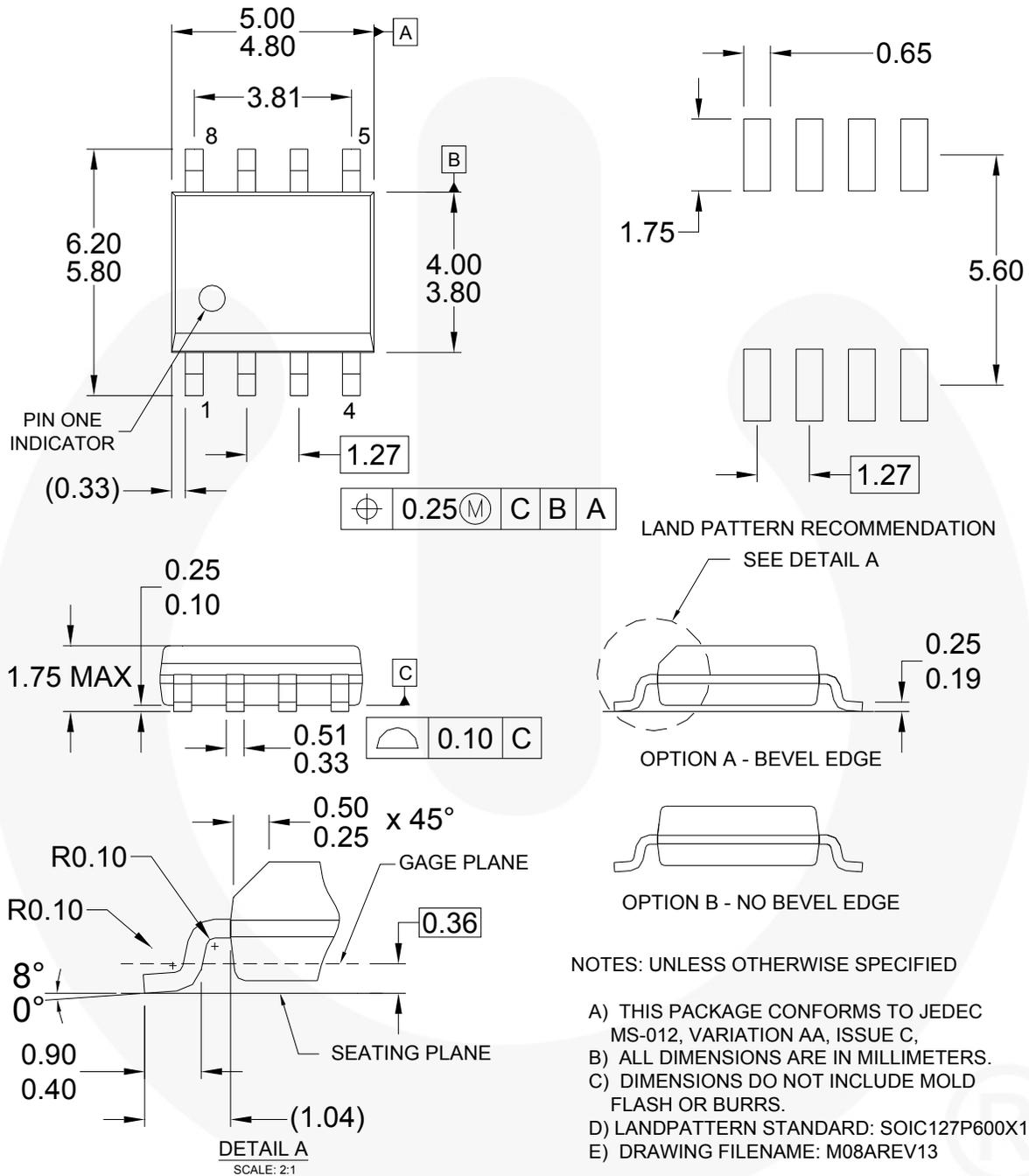
**Figure 14. 8-Lead Small Outline Integrated Circuit (SOIC)**
