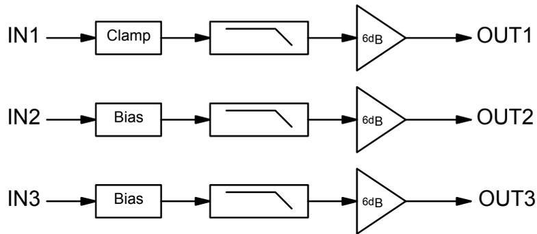
Figure 1. 7<sup>th</sup>-Order 30MHz Filter
