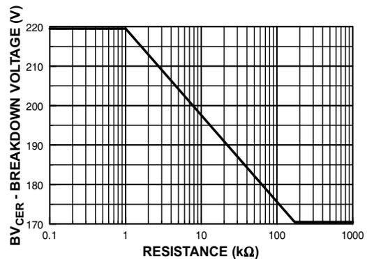
Figure 6. Collector-Emitter Breakdown Voltage with Resistance Between Emitter-Base
