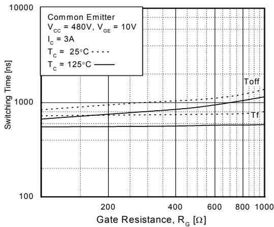
**Figure 10. Switching Loss vs. Gate Resistance**
