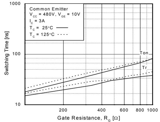
**Figure 9. Turn-Off Characteristics vs. Gate Resistance**
