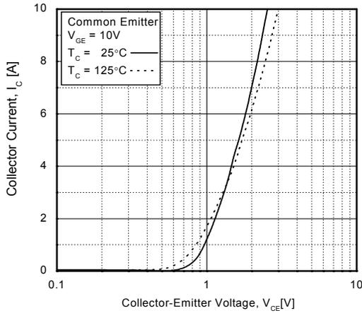
**Figure 4. Transfer Characteristics**
