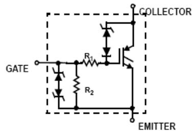
FGB3236\_F085 / FGI3236\_F085 320mJ, 360V, N-Channel Ignition IGBT
