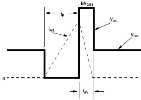
Figure 20. Energy Waveforms
