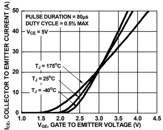
Figure 8. Transfer Characteristics
