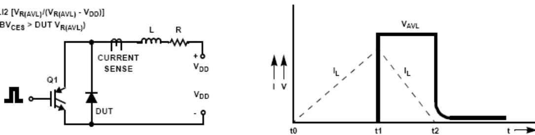
Figure 2. Unclamped Inductive Switching Test Circuit & Waveform
