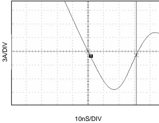
**Figure 12. FDS6690AS SyncFET body diode reverse recovery characteristic.**
