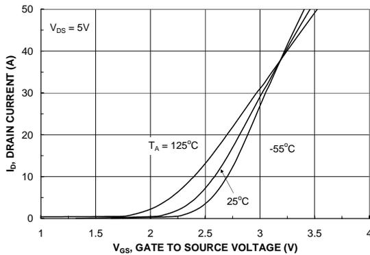
Figure 5. Transfer Characteristics.
