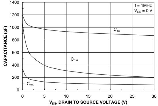
Figure 8. Capacitance Characteristics.
