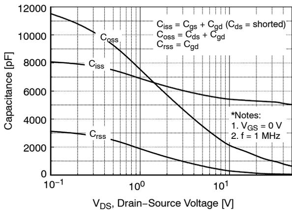
Figure 5. Capacitance Characteristics
