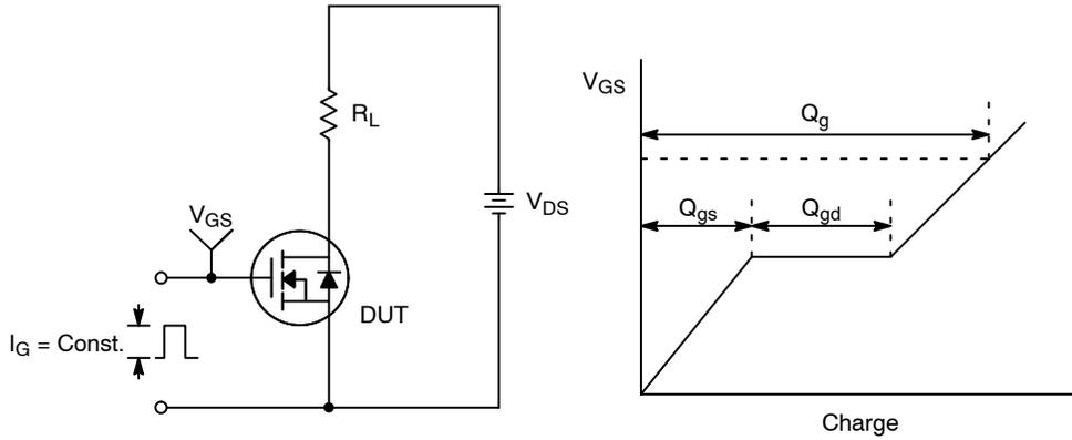
Figure 16. Gate Charge Test Circuit & Waveform
