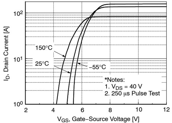
Figure 2. Transfer Characteristics
