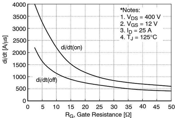
Figure 11. Typical Drain Current Slope vs. Gate Resistance
