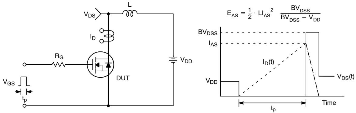
Figure 18. Unclamped Inductive Switching Test Circuit & Waveforms
