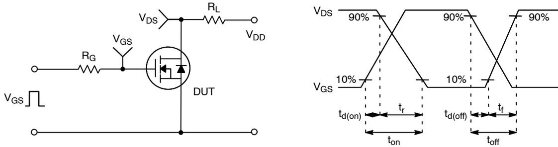
Figure 17. Resistive Switching Test Circuit & Waveforms
