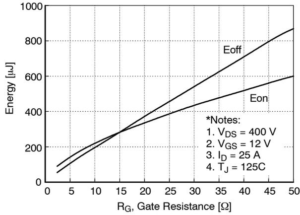
**Figure 13. Typical Switching Losses vs. Gate Resistance**
