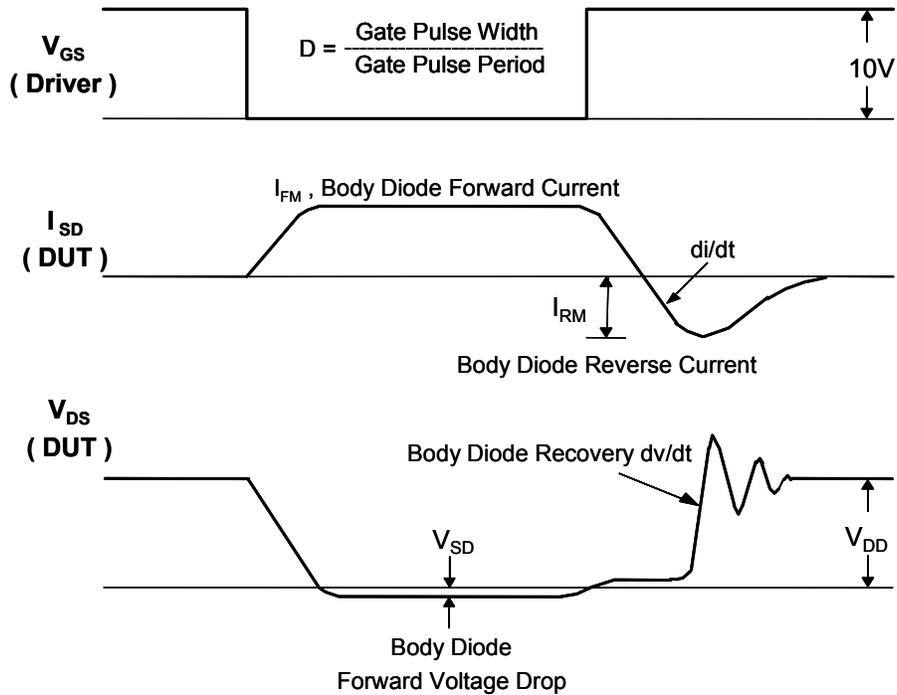
Figure 16. Peak Diode Recovery  $dv/dt$  Test Circuit & Waveforms
