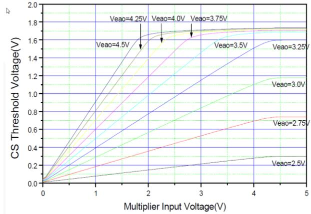
**Figure 4. Multiplier Input Voltage vs. Current Sensing Threshold**
