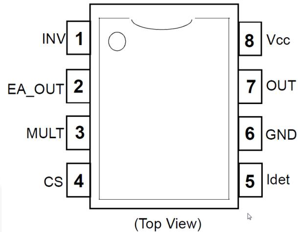
Figure 2. Pin Configuration
