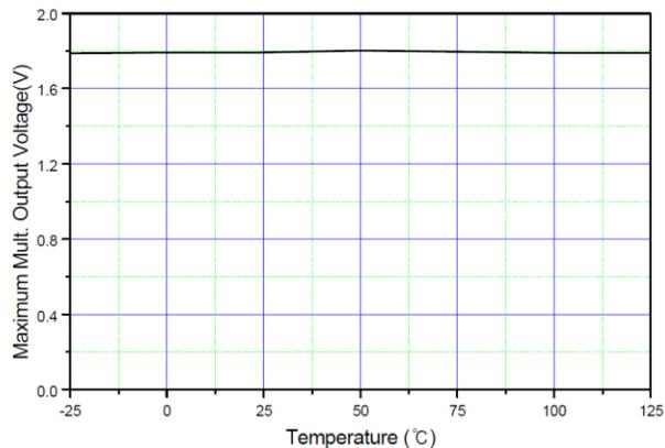
Figure 17. Maximum Multiplier Output Voltage vs. Temperature
