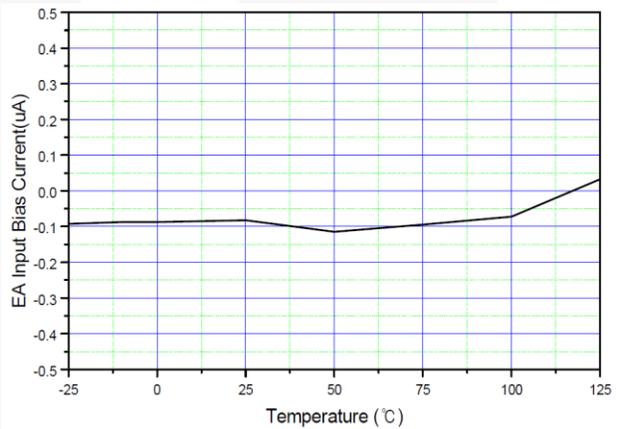
**Figure 12. Error Amplifier Input Bias Current vs. Temperature**
