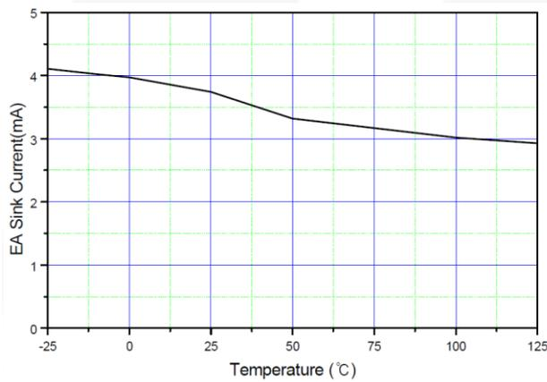
**Figure 11. Error Amplifier Sink Current vs. Temperature**
