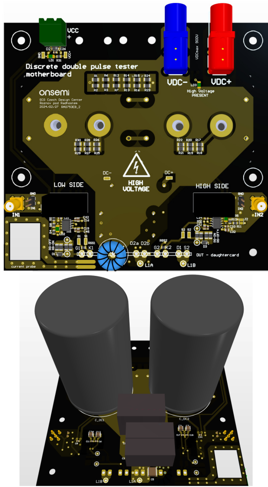
Figure 5. Mother Board TOP and BOTTOM View
