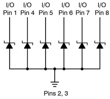
Note: Common GND – Only Minimum of 1 GND connection required
