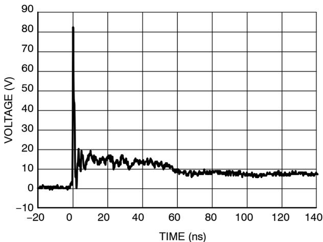
Figure 2. IEC61000-4-2 +8 kV Contact Clamping Voltage
