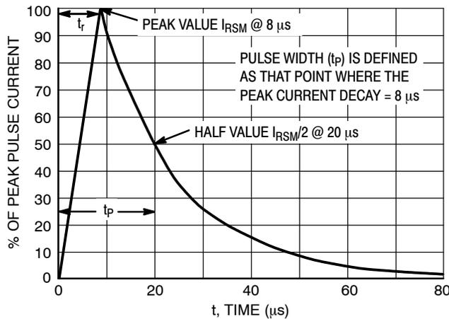
Figure 11. 8 X 20 μs Pulse Waveform
