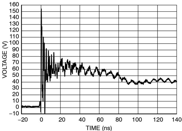
Figure 3. IEC61000-2-4 +8 kV Contact Clamping Voltage
