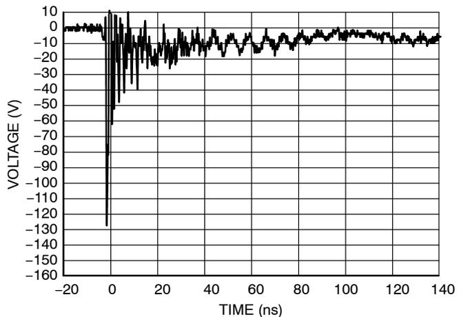
Figure 4. IEC61000-2-4 -8 kV Contact Clamping Voltage
