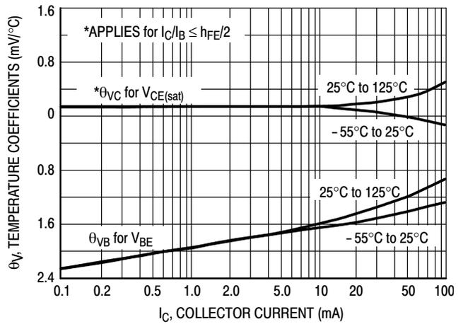
Figure 10. Temperature Coefficients
