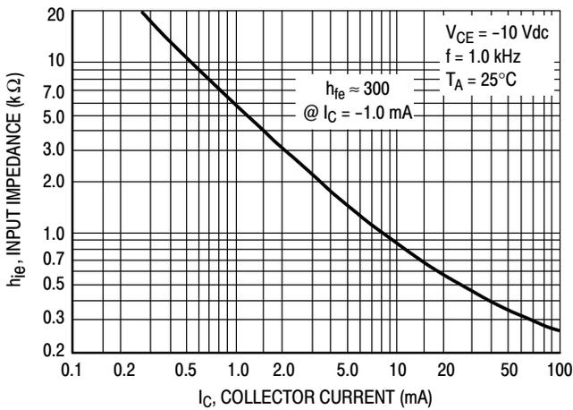
Figure 15. Input Impedance
