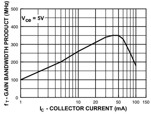
Figure 8. Gain Bandwidth Product vs. Collector Current
