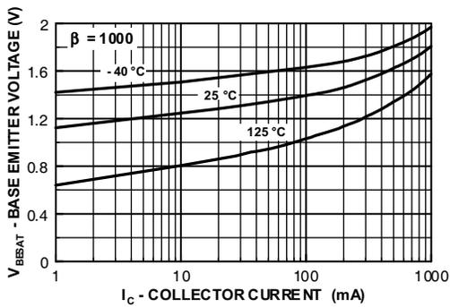
Figure 3. Base-Emitter Saturation Voltage vs. Collector Current
