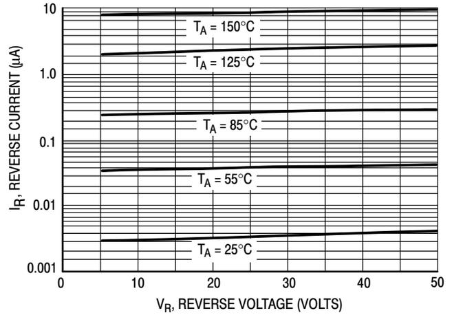
Figure 5. Leakage Current
