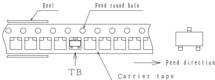
Those with one electrode terminal on the feed hole side.....TB
