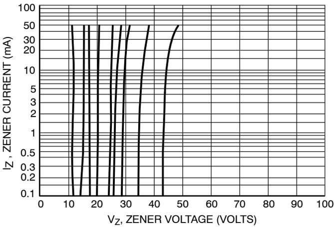
Figure 3.  $V_Z = 12$  thru 47 Volts
