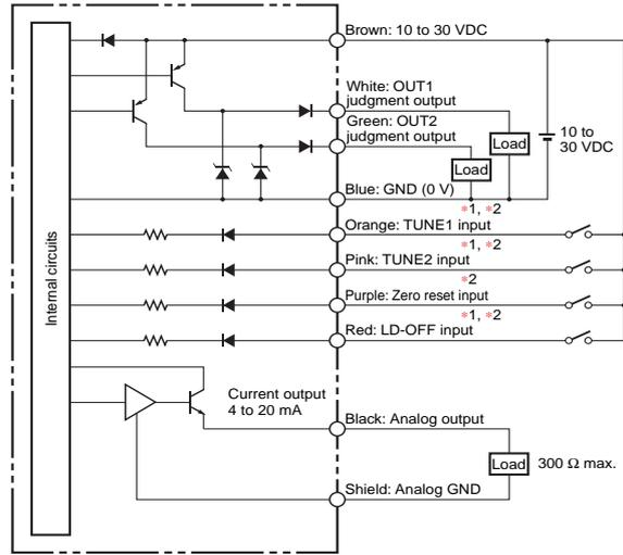
\*1. TUNE1 input: tuning external input for channel 1
