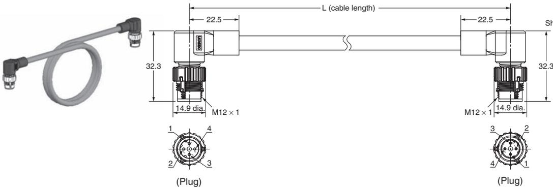
● Cable with Plugs on Both Ends (M12 Right-angle/RJ45)
