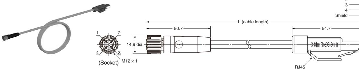
● Cable with Plug One End (M12 Right-angle)
