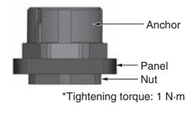
3. Attach the connector that you mounted to the PCB to the panel.
