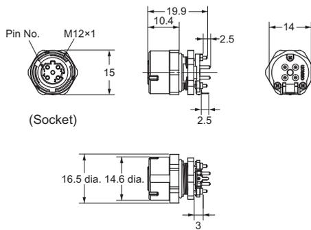
**Mounting Hole Dimensions (D Cut Structure)**
