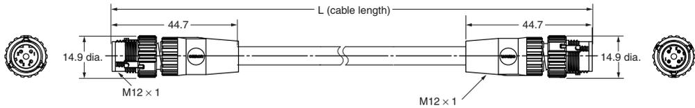
● Cable with Plugs on Both Ends (M12 Straight/RJ45)
