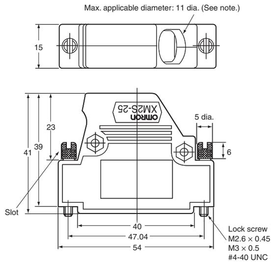
**Note:** The maximum applicable cable diameter is 9 dia if the cable clamp supplied is mounted facing the rear. Do not use a cable bushing in this case.
