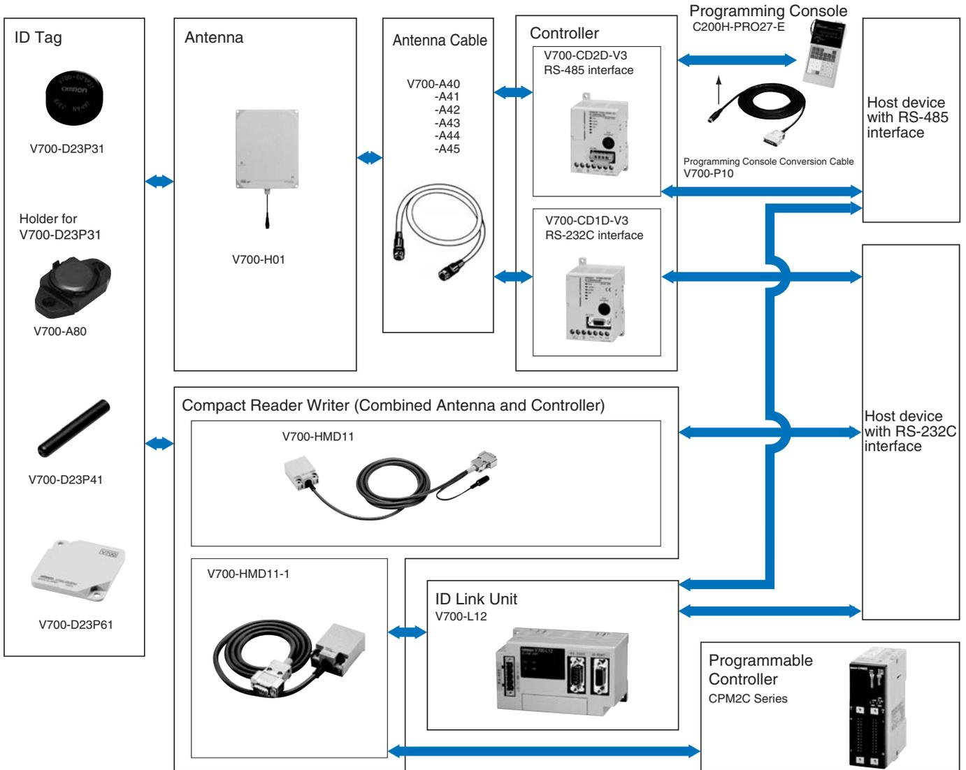
**Note:** The V700-CD1D-V3, V700-HMD11(-1), and V700-L12 all have different function and command structures.
