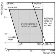
The above diagram is for standard conditions ( $+5^{\circ}$ C to  $+35^{\circ}$ C, 40% to 70%RH). Since the values vary depending on the operating environment conditions, contact your OMRON representative for further details.
