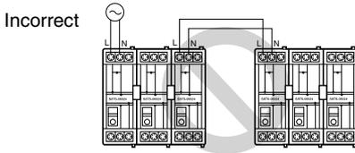
When Basic Blocks are linked together, it is necessary to wire the PE terminal of only one Basic Block, not all the Blocks.
