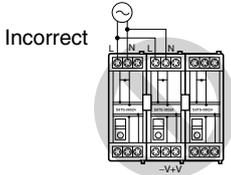
Do not cross-wire Blocks or wire between a Block and another device. If the current exceeds the rated current, Bus Line Connectors may be damaged.
