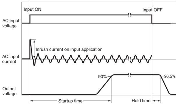
**Note:** The total inrush current of all of the Power Supplies will flow for parallel operation or backup operation. Sufficiently check the fusing characteristics of fuses and the operating characteristics of breakers and select fuses and breakers so that external fuses will not burn out or breakers will not operate due to inrush current.
