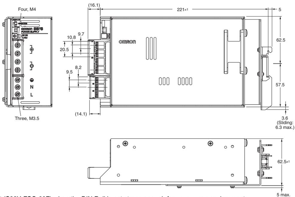
**Note:** Use a Front-mounting Bracket (S82Y-FSG-60F) when the DIN Rail is not strong enough for your usage environment.
