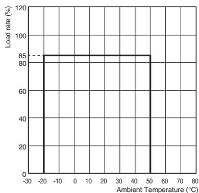
**Note:** At a voltage below 100 VAC, reduce the load at the rate of 1.3%/V.
