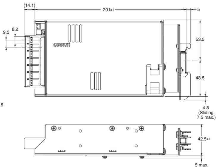
**Note:** Use a Front-mounting Bracket (S82Y-FSG-30F) when the DIN Rail is not strong enough for your usage environment.
