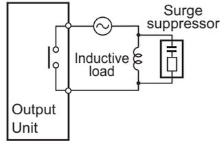
Connect a surge suppressor in an AC circuit.
