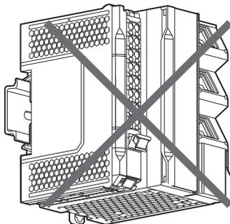
Mounting with the DIN Track Installed Vertically
