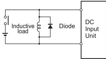
Connect a diode in a DC circuit.
