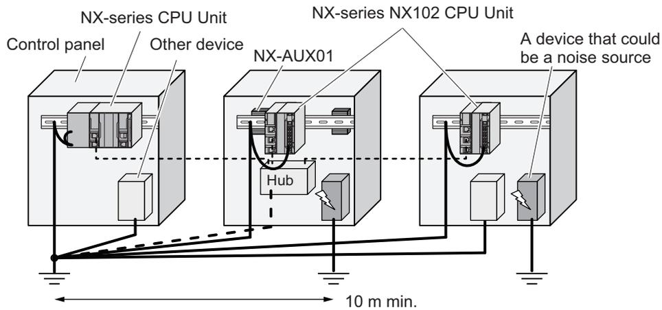
b. Installation by connecting devices and noise sources to a common earth electrode
