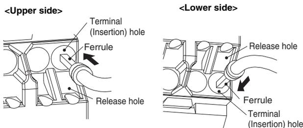
If a wire is difficult to connect because it is too thin, use a flat-blade screwdriver in the same way as when connecting stranded wire.
