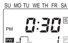
5. Press the **[WRITE]** Key. Set the time to 1:15 pm using the **[h]** and **[m/WD]** Keys.
