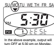
3. If the **WRITE** Key is pressed with the last setting for the week displayed, **End** is displayed for 2 s and then the Time Switch automatically returns to run mode.
