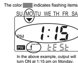
2. Press the **WRITE** Key. The display will change to the day and time of the next change in output status. (Continue pressing the **WRITE** Key to display the days and times for one week.)
