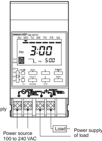
**Note:** 1. The Time Switch uses M3.5 terminals.
