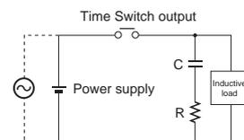
As a rough guide, the capacitor (C) and resistor (R) should have the following specifications:
