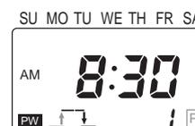
3. Press the **WRITE** Key. (If only the hour or the minute (but not both) is set, the operation setting time display will flash to indicate an error.)
