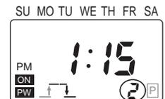
3. Press the **[CLR]** Key. (Both the ON and OFF settings are cleared with just one operation. If this operation is performed while output is ON, output stays ON until the Time Switch returns to run mode.)
