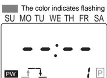
2. Press the **[TMR/Ⓟ]** Key to set the Time Switch for pulse-output operation. The **[P]** symbol flashes. (The Time Switch is set for timer operation at the time of delivery.)
