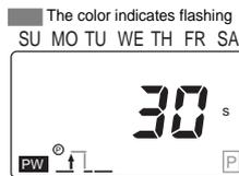
2. Change the pulse width to 20 s using **[m@WD]** Key.
