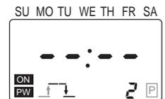
4. Press the **[MODE]** Key twice. The Time Switch will enter run mode and operation based on the new settings (i.e. without the cleared programs) will start.
