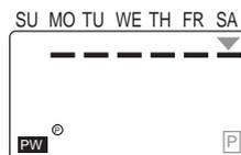
5. Press the **[MODE]** Key. The Time Switch will enter run mode and operation will start.
