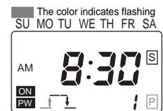
2. Press the **[CLR]** Key for 3 s min. The clearing process will be completed 3 s has elapsed. Output will turn OFF immediately.
