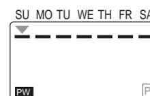
8. Move the **▼** symbol to Saturday using the **[d]** Key. Make the operation day indicator flash by pressing the **[WRITE]** Key. Move the present day indicator to Sunday using the **[d]** Key. Clear the operation day indicator by pressing the **[WRITE]** Key.
