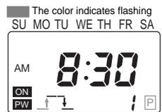
2. Change the ON time to 7:45 am using the **[h]** and **[m/WD]** Keys.
