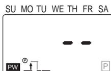
3. Set the pulse width to 30 s using the **[m/ⓂWD]** Key. (The pulse width can be set in the range 1 to 59 s or 1 to 60 min.)
