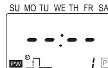
5. Set the ON time (the time when pulse-output operation starts) to 8:25 am using the **[h]** and **[m/ⓂWD]** Keys.
