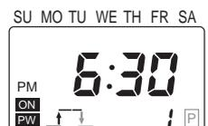
4. Press the **[MODE]** Key to enter operation date setting mode. The operation dates will be displayed. (Make changes, if necessary, using the **[d]** and **[WRITE]** Keys.)
