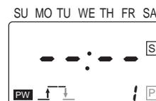
4. Set the OFF time for the specified day to 0:30 pm using the **[h]** and **[m/WD]** Keys.
