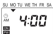
3. Press the **WRITE** Key. The colon will flash and the clock will start (from 0 s).
