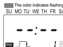
2. Set the ON time to 8:30 am using the **h** and **m@WD** Keys.
