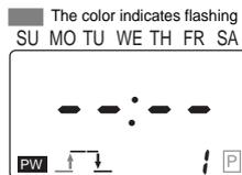
2. Press the **[SELECT]** Key. The **[S]** symbol will be displayed. Set the ON time for the specified day to 8:30 am using the **[h]** and **[m/WD]** Keys.
