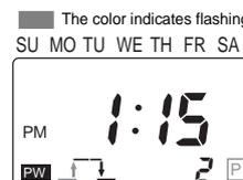
6. Press the **[WRITE]** Key. Set the time to 5:15 pm using the **[h]** and **[m/WD]** Keys.
