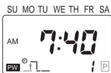
4. Press the **[MODE]** Key to enter operation date setting mode. The operation dates will be displayed. (Make changes, if necessary, using the **[d]** and **[WRITE]** Keys.)
