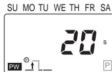
3. Press the **[WRITE]** Key. The ON time for program 1 will be displayed. (Make changes, if necessary, using the **[h]**, **[m@WD]** and **[WRITE]** Key.)
