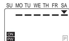
5. Press the **[MODE]** Key. The Time Switch will enter run mode and operation will start.
