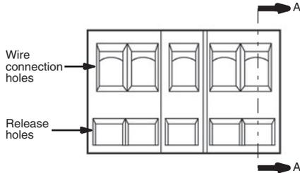
**Fig. 2 Wire Connection Holes and Release Holes**
