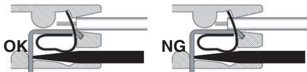
**2.** If the overall diameter of the wire is over 2.8 mm, it will be difficult to use double wiring.
