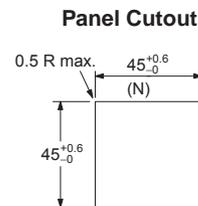
Note: The mounting panel thickness should be 1 to 5 mm.
