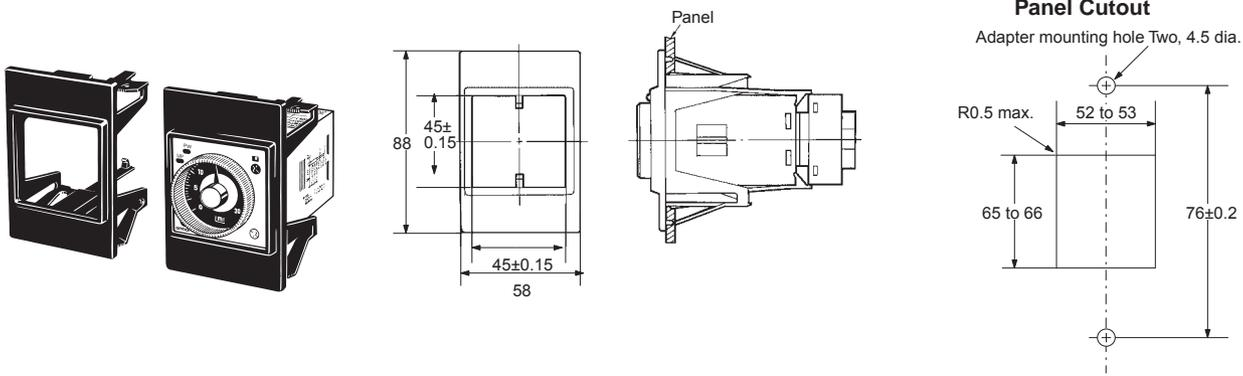
**Dimensions with Y92F-71 Flush Mounting Adapter**
