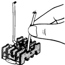
2. Connect the Timer to the Socket and press the tip of each hook by hand.
