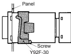
When using the US08, be sure to use 10.5-dia. max. multi-conductor cable or 3-dia. max. insulated stranded wire for wiring.
