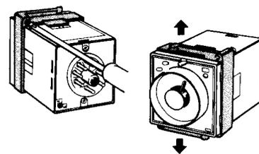
When the Y92F-30, Y92F-70, Y92F-71 Mounting Adapter is used, press the hook inwards with the thumb and index finger of both hands, and press the Timer towards the front side.
