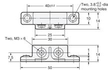
Note: Tighten each M3 screw of the terminal block to a torque of 0.59 N·m. max.
