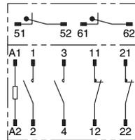
Note: The coil has no polarity.
