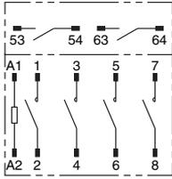
Note: The coil has no polarity.
