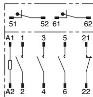
Note: The coil has no polarity.
