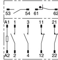
Note: The coil has no polarity.
