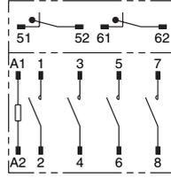
Note: The coil has no polarity.
