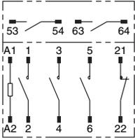
Note: The coil has no polarity.
