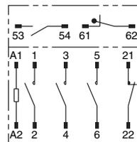
Note: The coil has no polarity.
