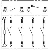
Note: The coil has no polarity.
