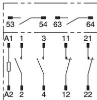
Note: The coil has no polarity.
