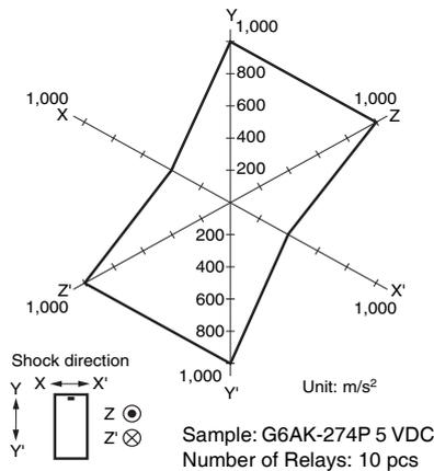
Test Conditions: Shock is applied in ±X, ±Y, and ±Z directions three times each with and without energizing the Relays to check the number of contact malfunctions.
