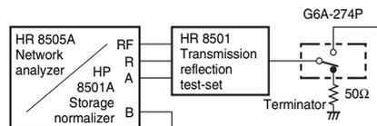
Terminals which were not being measured were terminated with 50 Ω.
