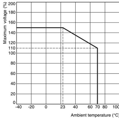
Note. The maximum voltage is the maximum voltage that can be applied to the relay cool.
