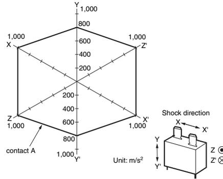
Test conditions: Shock is applied in  $\pm X$ ,  $\pm Y$ ,  $\pm Z$  directions three times each with and without energizing the Relays to check the number of malfunctions.
