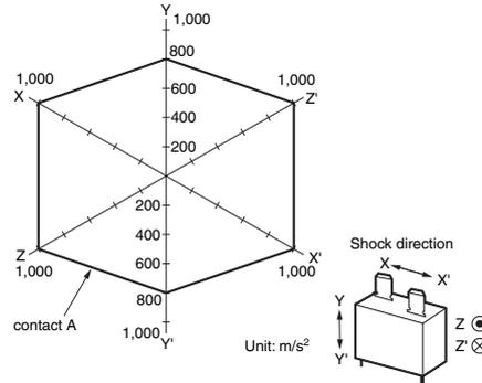
Test conditions: Shock is applied in  $\pm X$ ,  $\pm Y$ ,  $\pm Z$  directions three times each with and without energizing the Relays to check the number of malfunctions.
