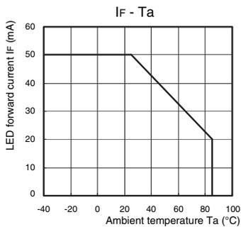
**Continuous load current vs. Ambient temperature**
