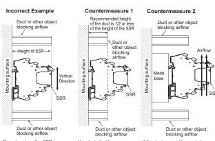
Do not enclose the SSR in a duct of the same height. It will interfere with the heat dissipation of SSR.
