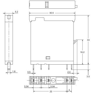
Terminal Arrangement/ Internal Connection Diagram (TOP VIEW)
