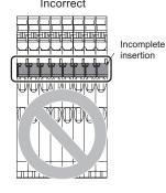
Incorrect installation Some terminals not inserted completely.
