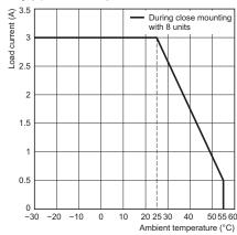
\*When eight or more are installed, install with 10 mm space between
