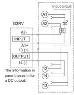
Equipped with a coil surge absorption circuit as standard.
