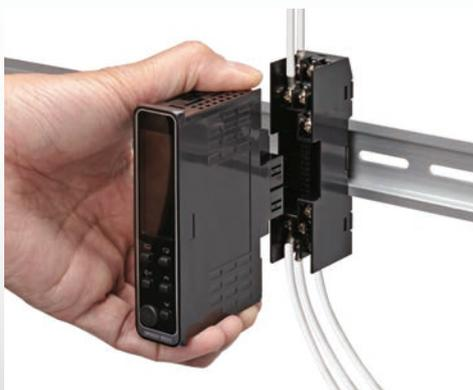
Removing from the Terminal Block
