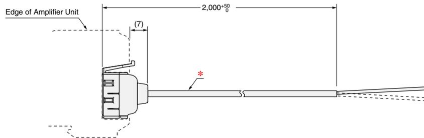
\* 2.6-dia. cable with 1 conductor, Standard cable length: 2 m (Conductor cross-section: 0.2 mm<sup>2</sup> (AWG24), Insulator diameter: 1.1 mm)
