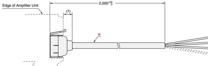
\* 4-dia. cable with 3 conductors, Standard cable length: 2 m (Conductor cross-section: 0.2 mm<sup>2</sup> (AWG24), Insulator diameter: 1.1 mm)
